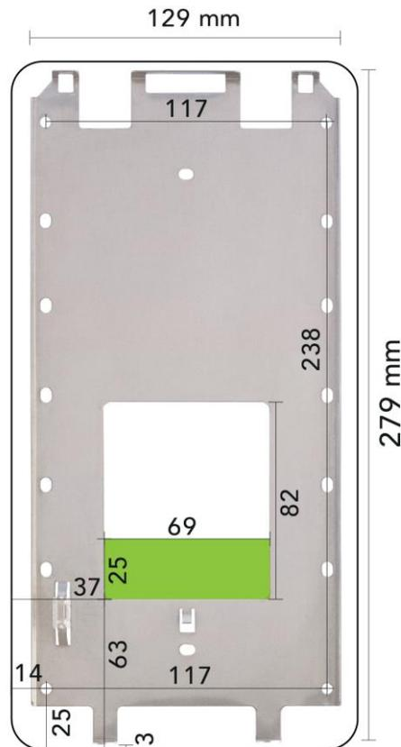
Front view of wall plate as mounted to the wall with outline of the reader. The bottom tabs face away from the wall. Lower edge of the reader is 3 mm lower than the lowest point of the plate.
