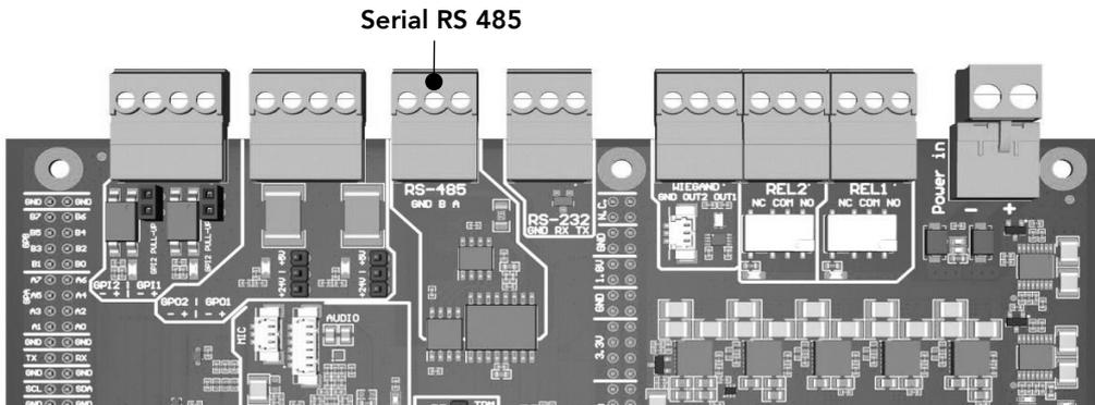
The device is equipped with an RS-485 serial interface on a detachable terminal block. There is no RS-485 bus termination resistor switch or socket on the device. Should such a resistor be required in the installation, please connect its leads to the wire terminal block.
