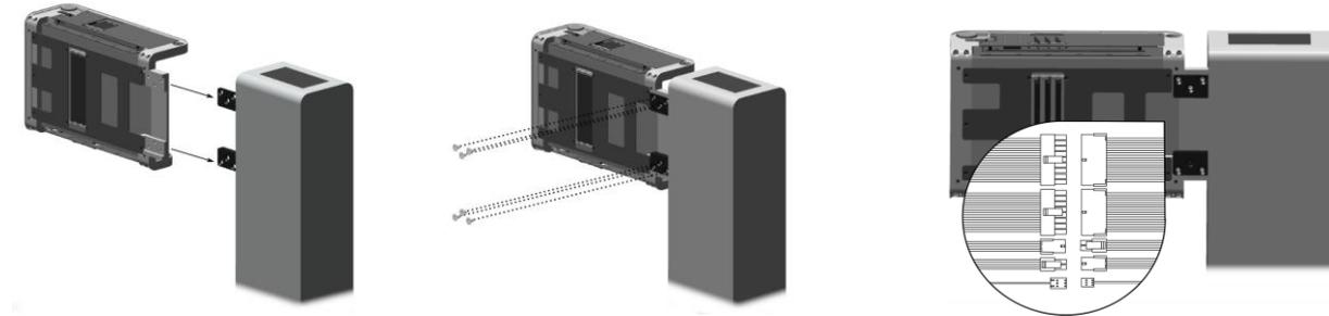
Third, connect the sensor cables to the pillar. There are 5 connectors coming from the back side of the sensor arm:
