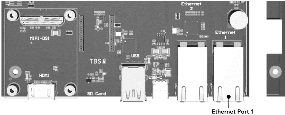
For connecting peripheral devices, the used cable should be of Cat5 or higher, and does not need to be crossed.
