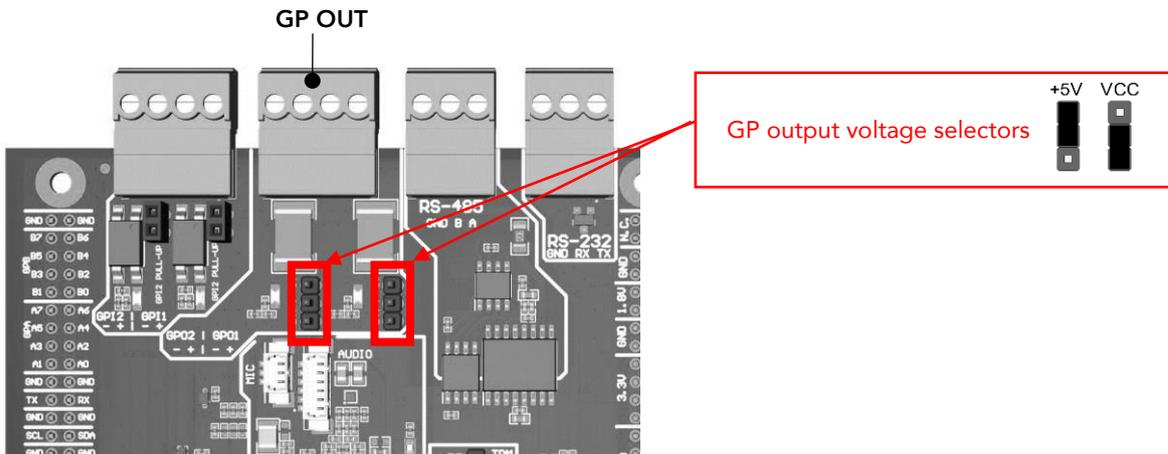
5 VDC level is set by default. To utilize the VCC voltage level, switch the jumper position of the respective voltage selector on the mainboard.
