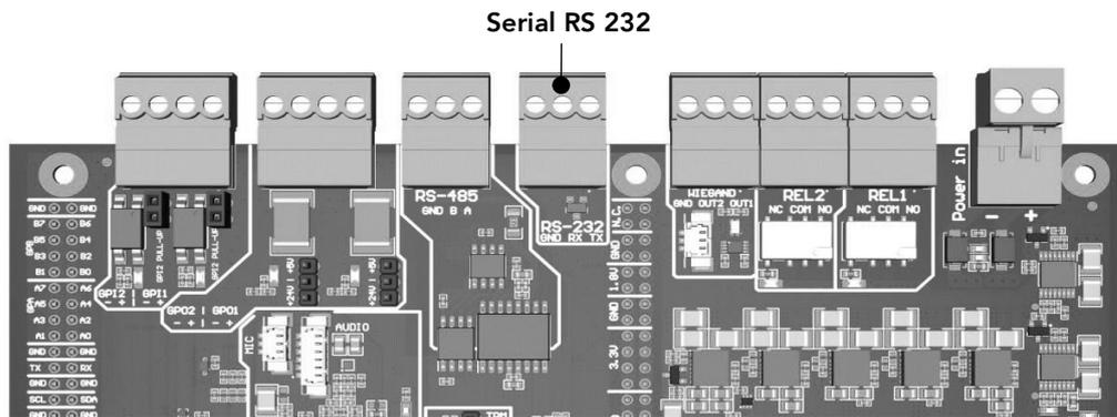
The device offers one serial RS-232 interface on a detachable terminal block to connect external controllers or other devices. The interface does not feature hardware flow control lines.
