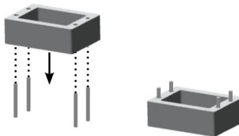
At this point, it is recommended to thread the cabling through the floor spacer. Route main power cable (optionally also a UTP network cable with RJ45 connector or other signalling cables for serial interfaces or relay switches) through the cable channel in the floor space. Inside of the main pillar you will need approx. 50 cm of power cable and approx. 75 cm of signal cables. The cables are wired to wire terminals once the main pillar is fixed to the bolts.
