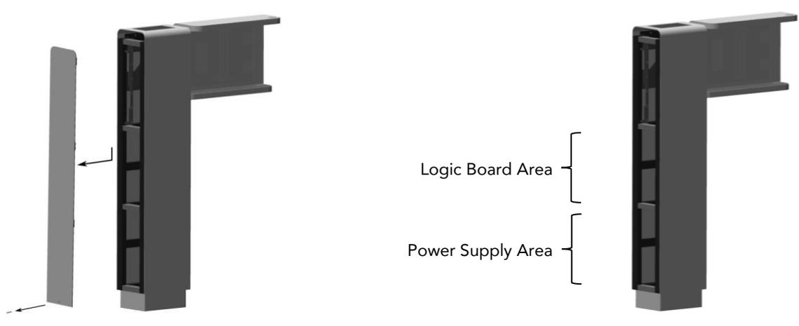
For simplified access, both the power supply and the main board are mounted on drawers that can be pulled out. To remove a drawer, first remove its securing screw. The drawers are designed such that they allow for servicing of parts even when not fully pulled out.
