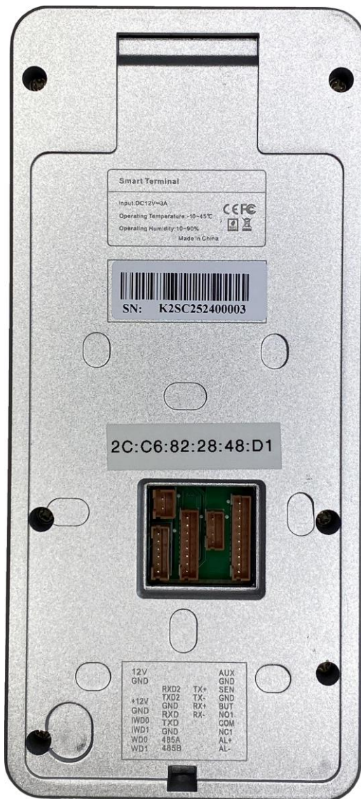
Backside view with wire connection pass through (power, LAN, serial)
