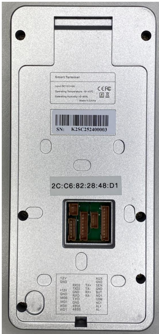
Backside view with wire connection pass through (power, LAN, serial)
